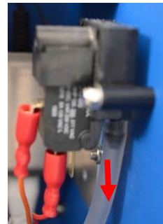
Pull tube off pressure switch
